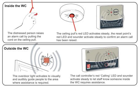
**Note:** The call controller's on-board relay will also activate when an alarm call is made and any external equipment connected to the relay contacts will operate as configured.
